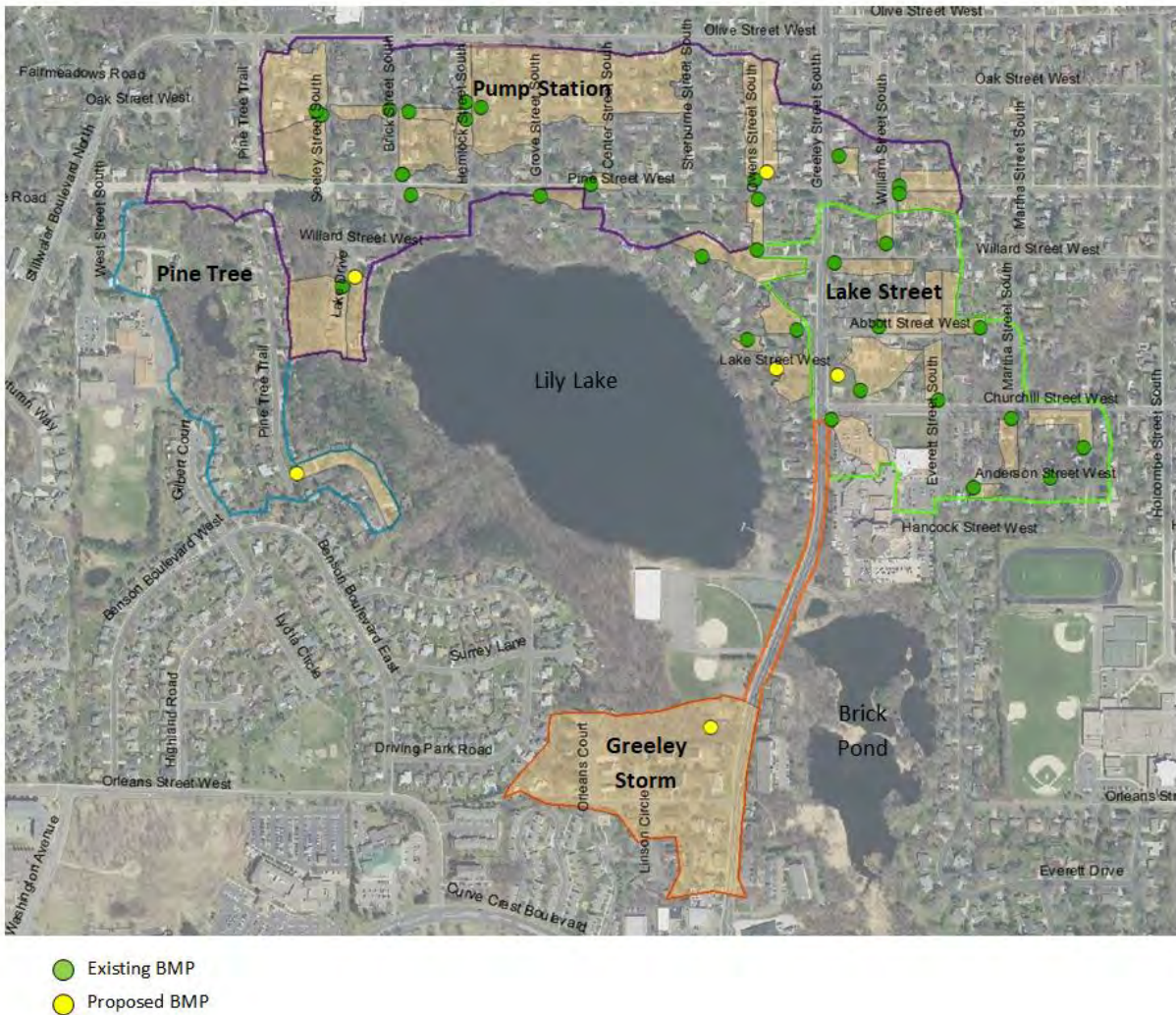
Figure 10. Water quality BMPs and their catchment boundaries within the direct drainage area of Lily Lake
