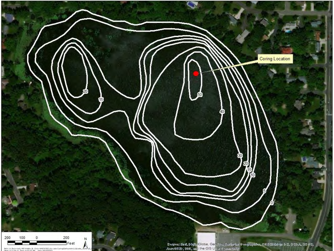
Figure 1. Bathymetry contours (ft.) and sediment coring location on Lily Lake. Note that the lake contours were georeferenced from an image and are added just for reference.
